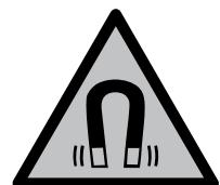
**Keep the magnetic accessories away from implants and other medical devices, e.g. pacemakers or insulin pumps.** The magnets in the accessories generate a field that can impair the function of implants and medical devices.
