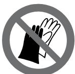
**Do not wear gloves when taking measurements and make sure that you are properly earthed.** If you are not properly earthed, the material identification of "live" wires may be impaired.
