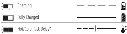
\*The red light will continue to blink, but a yellow indicator light will be illuminated during this operation. Once the battery pack has reached an appropriate temperature, the yellow light will turn off and the charger will resume the charging procedure.
